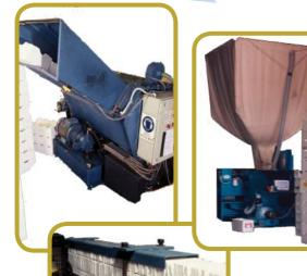
4. The EPS is granulated and stored in a hopper before being compacted.
