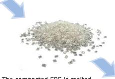
5. The compacted EPS is melted, pelletised and converted into General Purpose Polystyrene (GPPS)
