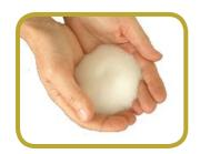
1. Tiny grains of styrene are expanded using steam. The expanded beads are then moulded into shapes or large blocks depending on the application.
